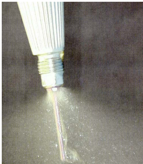
Figure 3. Atomization of irrigation fluid at tip (horn) shoulder.
